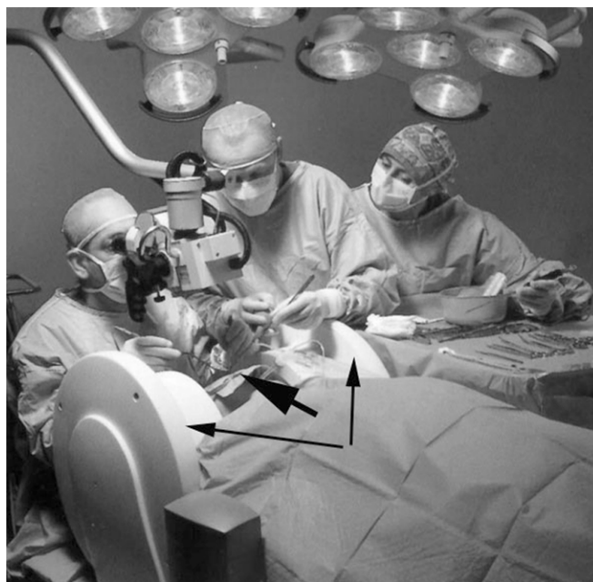
Figure 4. A small-scale intraoperative MRI scanner developed by Odin Technologies (Yokneam, Israel) that can be used on demand in a regular operating suite. The long arrows indicate the separated discs of the magnet. The short arrow indicates the position of the patient's head during the operation
