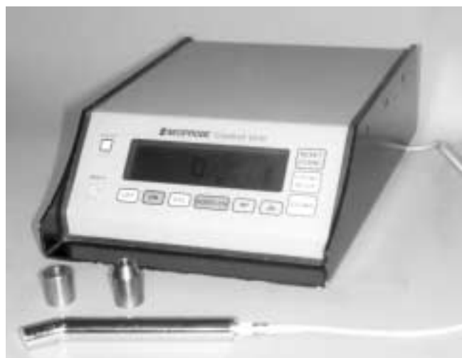
Figure 1. Gamma detecting probe with two types of collimators for intraoperative parathyroid detection.
